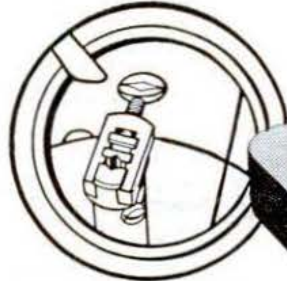
Steel universal chuck holds all blades, files, and sanding attachments.
